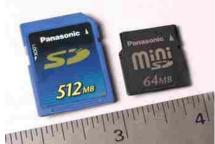
MiniSD card for cellphones, MP3 players, digicams. The miniSD card is both electrically and software compatible with the existing SD standard. It uses the same SD interface, including security features for content protection (CPRM—Content Protection Rights Management) as the standard SD card. The miniSD card is 21.5 millimeters (mm) long, 20 mm wide and 1.4 mm thick, and occupies a footprint of 430 square mm and volume of 602 cubic mm.
